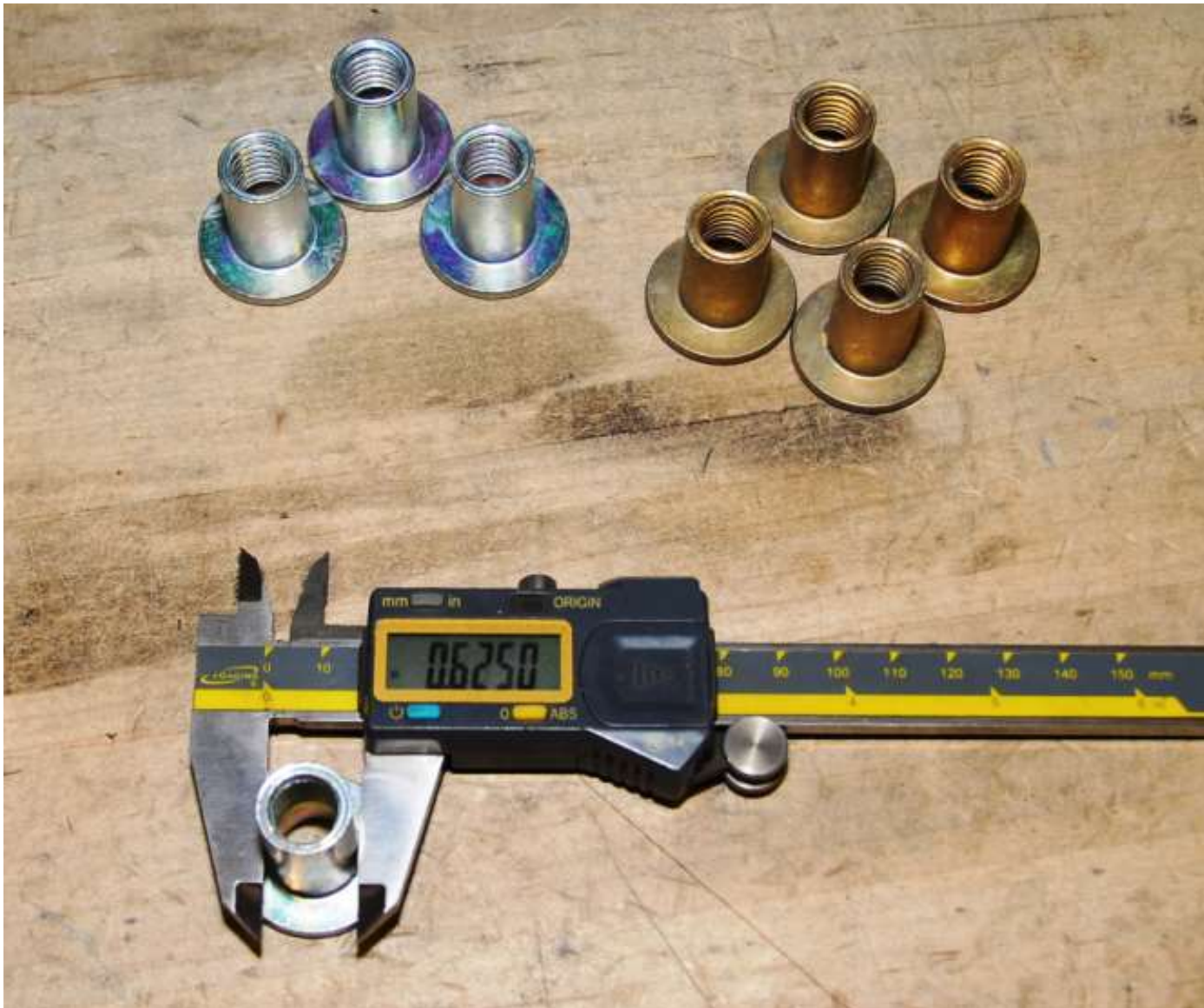
Shown below are the OEM Nutserts for the belly skid in both metric (goldish color) and SAE (silver color)
